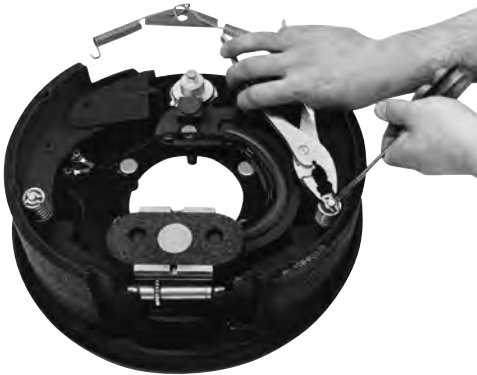
Figure 55 - Removing Shoe Hold Down Assemblies
