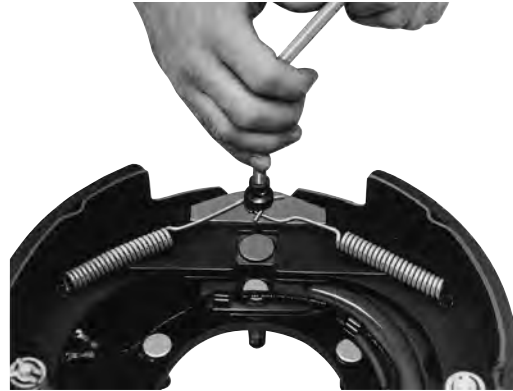
Figure 17 - Removing Shoe Return Springs
